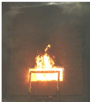
Figure 4: Fire emitting from the test window
