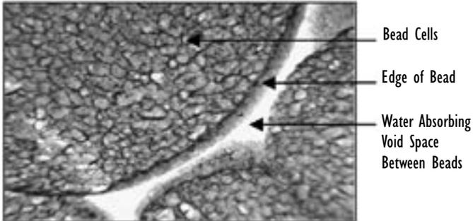
Compare XPS (Fig. 1) to EPS (Fig. 2). Because of the homogeneous cross section of XPS, very little water is absorbed into the cell structure. "Closed cell" means very little R-value reducing water will be absorbed into the insulation board. The XPS extrusion process produces that closed cell structure. The EPS expansion process does not, therefore, EPS should be considered an open void structure.
