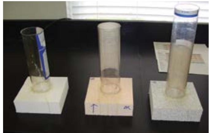
**Figure 4b: EPS Water Absorption via Wicking**
