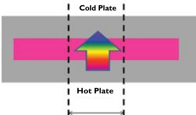
R-value is measured through the center section of the sample
