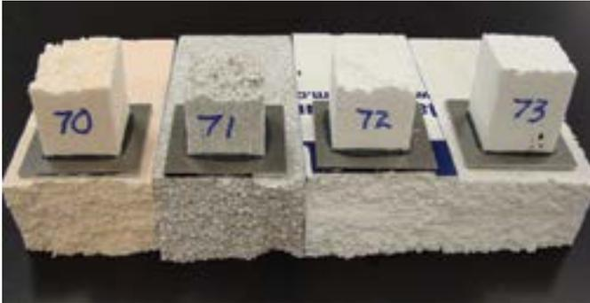
**EPS Sample ID:** Sample 70 is ASTM C578 Type II, density 1.64 pcf; 71 was identified as Type IX by its manufacturer; but measured 1.62 pcf which is a high density version of Type II; 72 is Type XIV, 2.55 pcf; 73 is Type XV, 2.71 pcf
