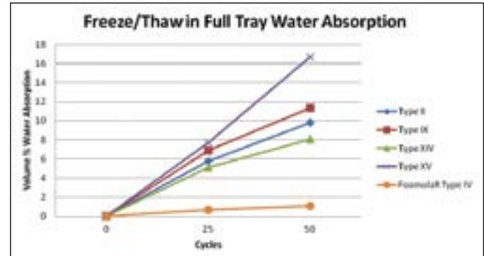
Samples fully submerged in water during freezing and thawing.
